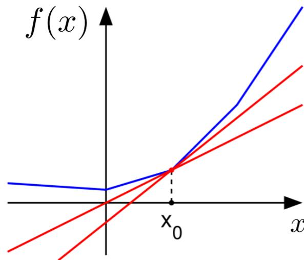
Sous-gradient (subgradient)  $\partial f(x_0)$
